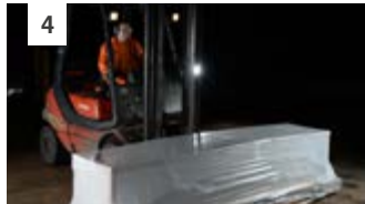
4 Pallets are shrink wrapped for protection, and clearly labelled with location details and handling instructions.
