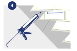
Use lead sealant to point the flashing and give it a professional finish
