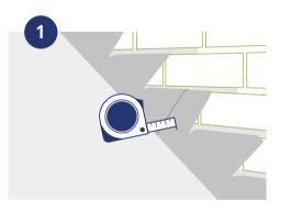
Measure the chase joint. For smaller joint up to 18mm use the fixing clip. For larger joints from 16mm – 26mm use the flashing clip
