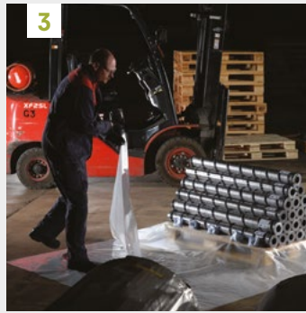
3 We place silica gel (to absorb moisture) on the pallet and wrap the lead for the first time
