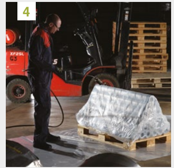
4 The lead sheet is shrink-wrapped to keep any moist out
