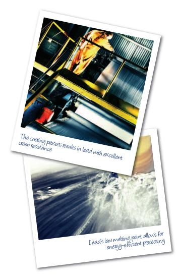
Through a computerised process, controlling the depth of immersion and the speed of rotation of the drum, Midland Lead is able to produce lead sheet conforming to customers' specifications - thicknesses between 0.44 up to 3.55 mm.
